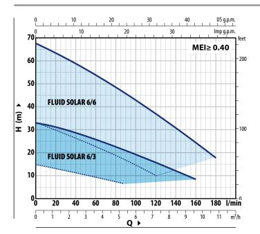
Performance curves comply with EN ISO 9906 Grade 3B tolerance limits.
